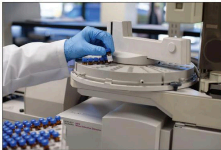
Gas chromatography is used to analyze terpenes and residual solvents in cannabis extracts.
